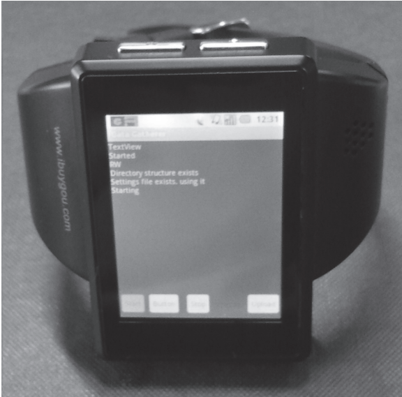
Fig. 2. The Z1 smartwatch used in the USEFIL project to monitor activity.
