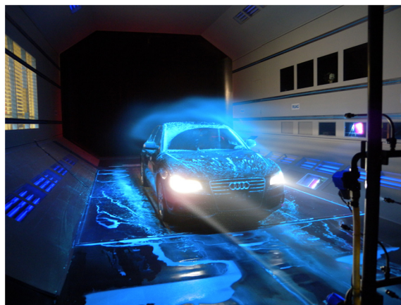
Figure 8. Typical wind tunnel spray grid experiment. Source: photograph courtesy of RUAG.
