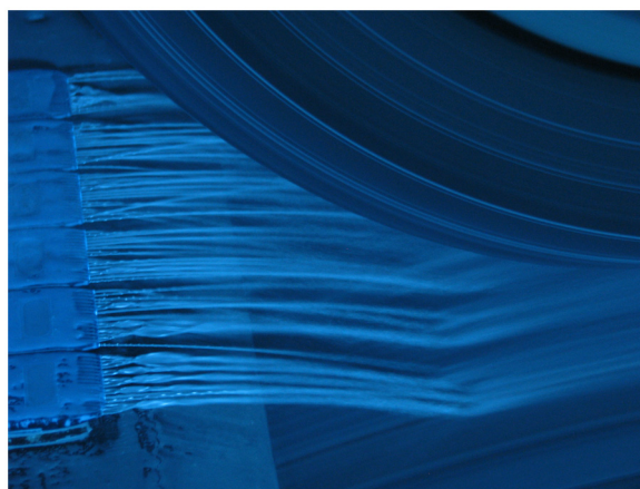
Figure 9. Water and UV dye introduced on to a dynamometer roller in the FKFS thermal wind tunnel to simulate the tyre spray. Source: photograph courtesy of FKFS.
