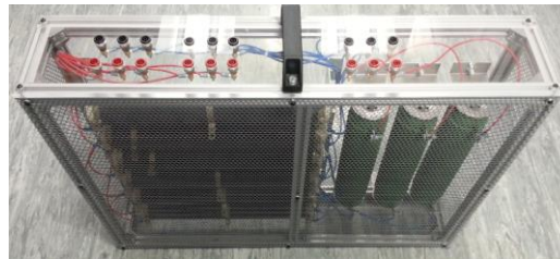
Figure 5:23: Resistive Load Bank
