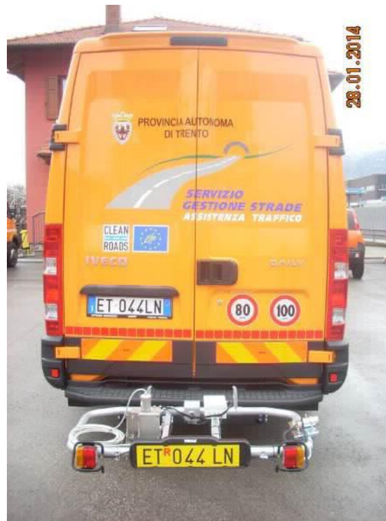
Figure 2. Thermal mapping vehicle.
