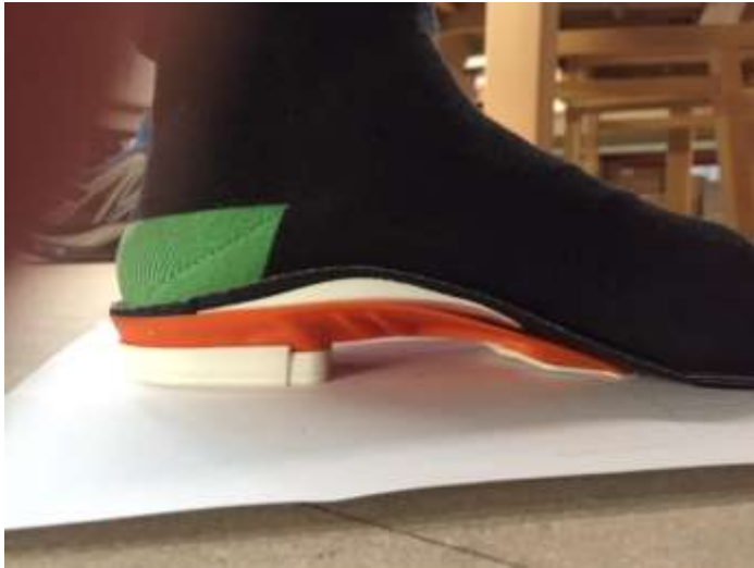
Fig 26: Person stood on vector orthotic with heel and mid foot piece attached (Parker, 2016)
