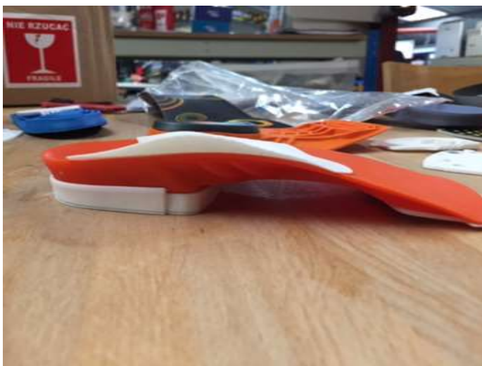
Fig 28: Orange vector with 3D printed front, mid and heel pieces side View (Parker, 2016)
