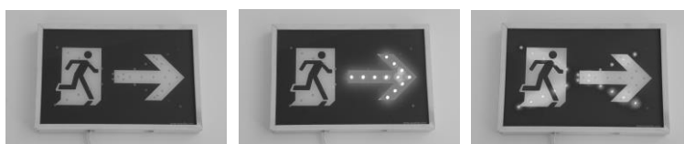
Fig. 1. The standard exit sign (left), the dynamic signage concept (middle) and the negated signage concept (right).
