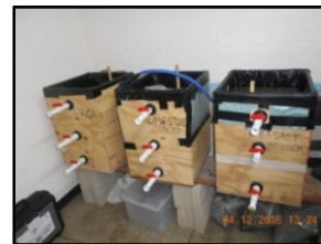
Fig. 4. Completed pavement plywood rigs.
