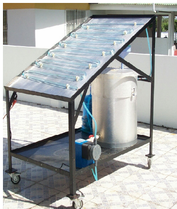
Fig. 5. Solar photoreactor in operation, Trinidad, West Indies.
