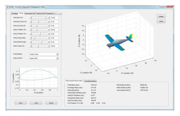
Figure 11 Aircraft Virtual Prototyping Tool
