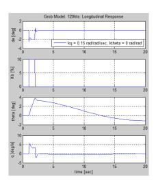
Figure 10 Example Pitch Rate Response for Controller Design
