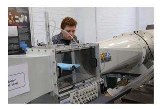
Figure 8 AF100 Demonstrator Wind Tunnel
