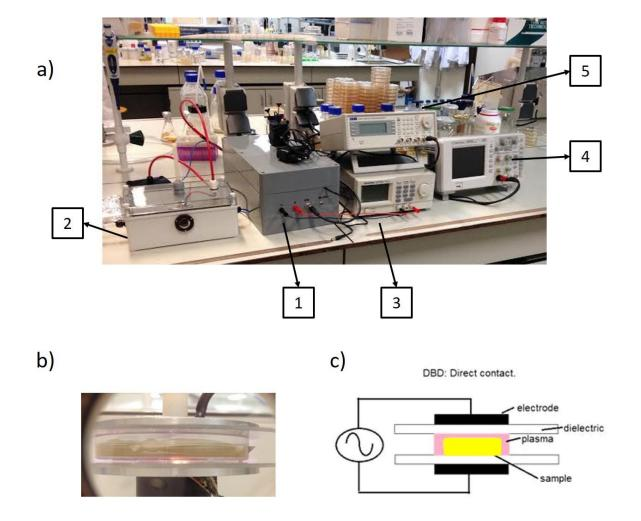
Figure 2: (a) the CAP set up: (1) plasma power source, (2) Dielectric Barrier Discharge reactor (22.5 cm x 13.5 cm x 10 cm), (3) DC power supply, (4) oscilloscope and (5) function generator. (b) DBD electrode inside reactor (electrode: diameter 5.5 cm, dielectric: 7.5 cm) petri dish containing sample: petri dish with diameter 5 cm). (c) Schematic representation DBD electrode with sample.
