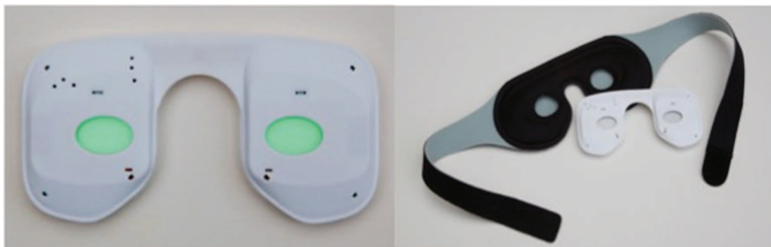
Figure 1 Principal components of OLED sleep mask. Left panel: plastic pod containing OLED light source delivering light at 504 nm peak for a maximum of 8 h with dose delivery sensor. Right panel: soft cushioned fabric mask that houses the plastic pod.
