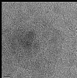
Fig.1: Micrograph showing atomic scale crystalline domains in semiconducting ZnO grown by ALD.
