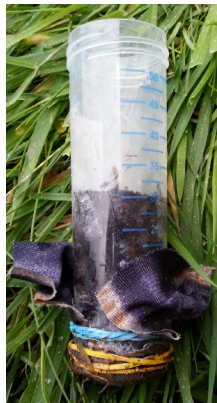
(b) Filled with soil and bottom drain and no cap
