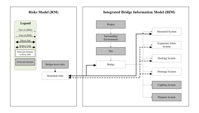
Figure 12 Linkage between structural risks and bridge information model
