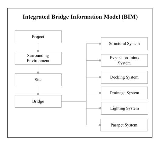
Figure 9 Separation of an integrated bridge information model
