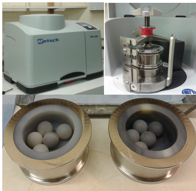
Figure 4.10: Planetary Ball Mill Instrument used to prepare the samples for XRF analysis.
