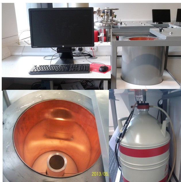
Figure 3.12: BEGe detector, shielding system and cryostat.
