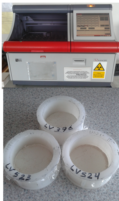
Figure 4.11: The X-ray fluorescence system and some of the analysed samples.
