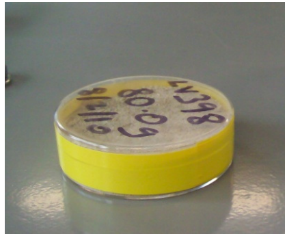
Figure 5.4: A prepared sample filling in a cylindrical container and sealed.
