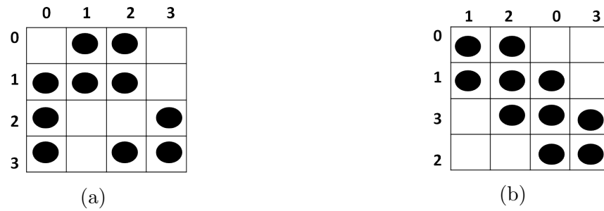
FIGURE 1.1: 2D Banding Example: (a) original matrix and (b) original matrix with the rows and columns reordered to reveal a banding
