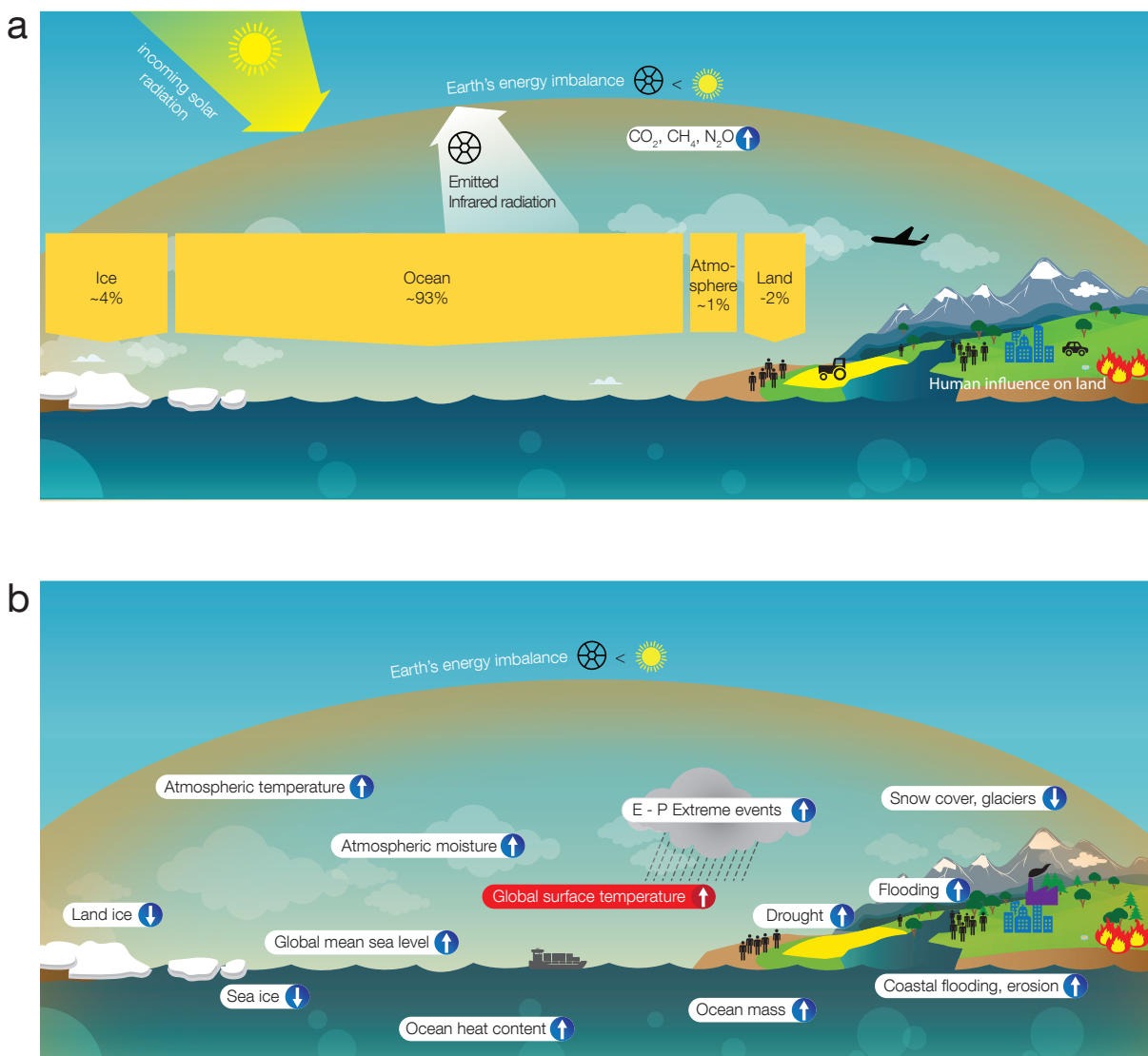
Figure 1.6 Schematic representations of: a the flow and storage of energy in the Earth's climate system. The global ocean is the major heat reservoir, with \sim 93\% of EEI stored there. The rest goes into warming the land, atmosphere and melting ice and snow. And, b the consequences of EEI and the resulting global warming caused by human activities that is leading to rising surface temperature, ocean heat content, ocean mass, global mean sea level, atmospheric temperature and moisture, drought, flooding and erosion, increases in extreme events, and evaporation – precipitation (E–P), plus a reduction in ice sheets, glaciers, sea-ice and snow cover. Redrawn and modified after von Schuckmann et al. (2016).
