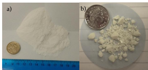
Figure 2. (a) Large scale batch synthesis (>10 g) of CC3 yields a pure polycrystalline material. (b) Large, millimeter-sized single crystals suitable for single crystal X-ray diffraction can also be isolated directly from reaction mixtures.
