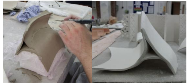
Figure 6: Forming the component out of clay slabs
