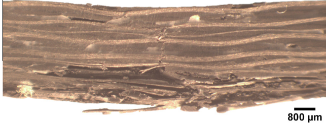
Fig. 3. Optical micrograph showing the damaged section of the n=3/4 panel following test at a scaled energy of E=97.22n^3 Joules.
