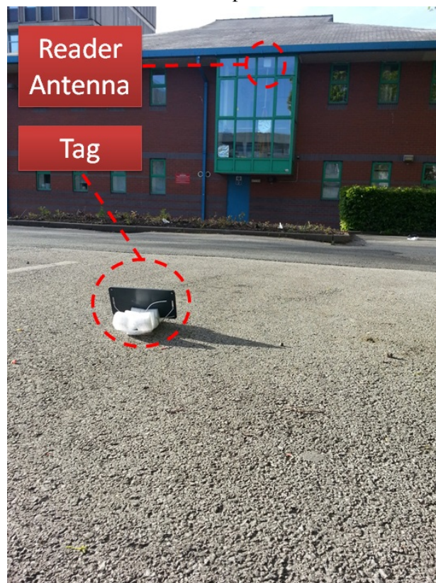
(b) Omni Dura 3000 passive tag on the asphalt and oriented to the reader antenna.
