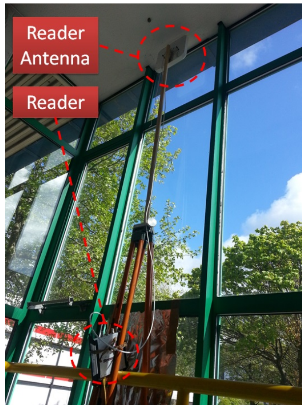
(a) RFID reader and antenna connected and positioned towards an outdoor parking lot.
