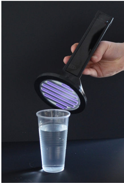
Figure 2. Portable air plasma device operating in a continuous mode of operation at 10 W dissipated power.
