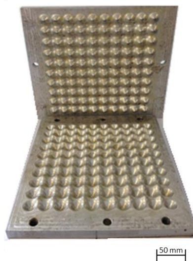
Figure 3.7 Spherical roof countoured mould.
