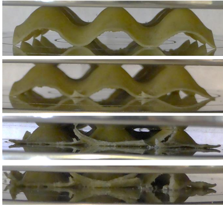
Figure 4.16 Crushing process in the GFRP spherical roof contoured core.
