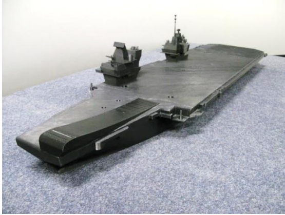
Figure 11: Fully assembled QEC 1:202 scale (1.4m length) model
