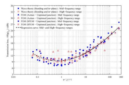
**Figure 7.** L-junctions  $(-10\lg(\gamma_{12}) \text{ versus } \psi/\chi)$ . Comparison of wave theory and FEM in (a) the low-frequency range and (b) the mid- and high-frequency ranges.
