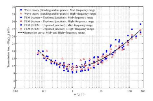
**Figure 8.** T-junctions  $(-10\lg(\gamma_{12}) \text{ versus } \psi/\chi)$  – transmission around the corner. Comparison of wave theory and FEM in (a) the low-frequency range and (b) the mid- and high-frequency ranges.
