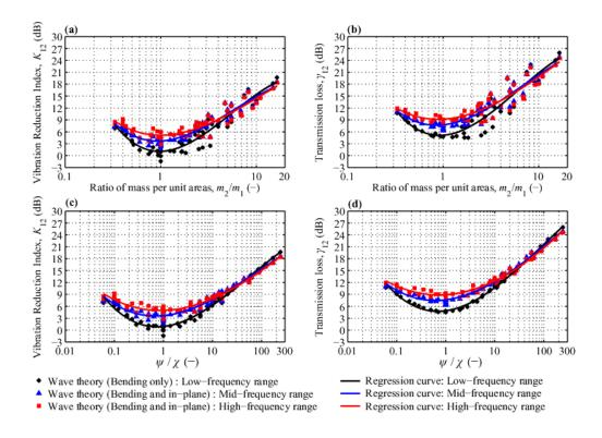
**Figure 2.** Comparison of L-junction data calculated using wave theory. (a)  $K_{12}$  versus M, (b) -  $10\lg(\gamma_{12})$  versus M, (c)  $K_{12}$  versus  $\psi/\chi$ , (d) - $10\lg(\gamma_{12})$  versus  $\psi/\chi$ .
