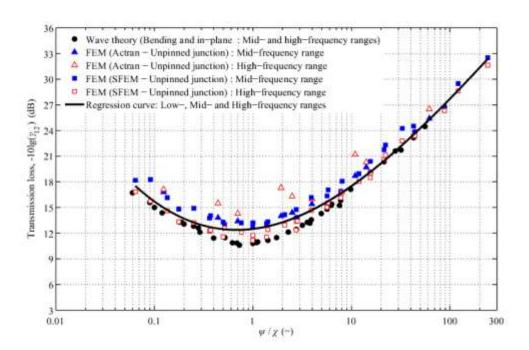
**Figure 10.** X-junctions  $(-10\lg(\gamma_{12}) \text{ versus } \psi/\chi)$  – transmission around the corner. Comparison of wave theory and FEM in (a) the low-frequency range and (b) the mid- and high-frequency ranges.
