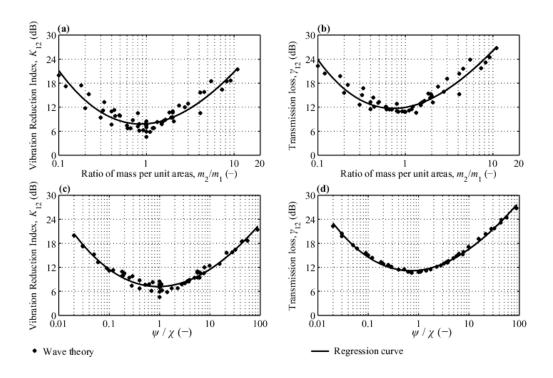
**Figure 4.** Comparison of X-junction data (transmission around the corner) calculated using wave theory. (a)  $K_{12}$  versus M, (b)  $-10\lg(\gamma_{12})$  versus M, (c)  $K_{12}$  versus  $\psi/\chi$ , (d)  $-10\lg(\gamma_{12})$  versus  $\psi/\chi$ .
