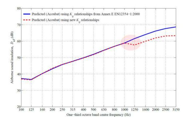
**Figure 13.** Comparison of predicted sound insulation using existing and new  $K_{ij}$  relationships to illustrate the existence of a step from 1kHz to 1.25kHz.
