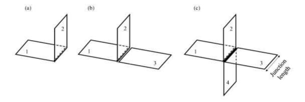
Figure 1. Junction types: (a) L-junction, (b) T-junction (c) X-junction.
