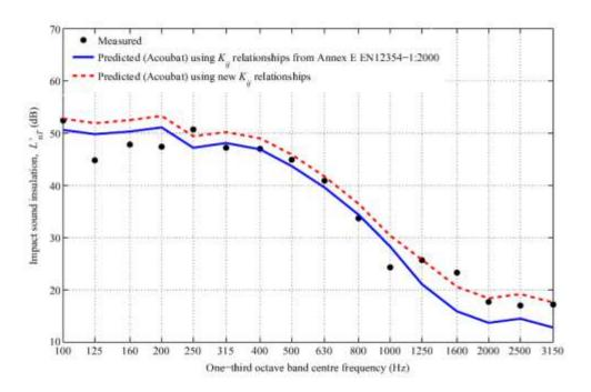
**Figure 12**. Comparison of measured and predicted sound insulation using existing and new  $K_{ij}$  relationships for a typical concrete building: (a) airborne (vertical configuration) sound insulation, (b) impact (horizontal configuration) sound insulation.
