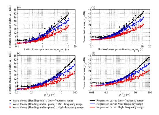
**Figure 6.** Comparison of X-junction data (transmission across the straight section) calculated using wave theory. (a)  $K_{13}$  versus M, (b)  $-10\lg(\gamma_{13})$  versus M, (c)  $K_{13}$  versus  $\psi/\chi$ , (d)  $-10\lg(\gamma_{13})$  versus  $\psi/\chi$ .
