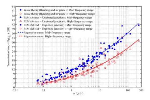
**Figure 11.** X-junctions  $(-10\lg(\gamma_{13}) \text{ versus } \psi/\chi)$  – transmission across the straight section. Comparison of wave theory and FEM in (a) the low-frequency range and (b) the mid- and high-frequency ranges.
