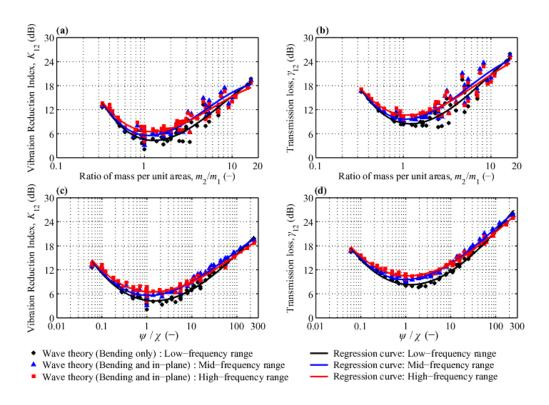
**Figure 3.** Comparison of T-junction data (transmission around the corner) calculated using wave theory. (a)  $K_{12}$  versus M, (b)  $-10\lg(\gamma_{12})$  versus M, (c)  $K_{12}$  versus  $\psi/\chi$ , (d)  $-10\lg(\gamma_{12})$  versus  $\psi/\chi$ .
