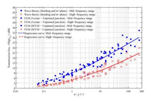
**Figure 9.** T-junctions  $(-10\lg(\gamma_{13}) \text{ versus } \psi/\chi)$  – transmission across the straight section. Comparison of wave theory and FEM in (a) the low-frequency range and (b) the mid- and high-frequency ranges.
