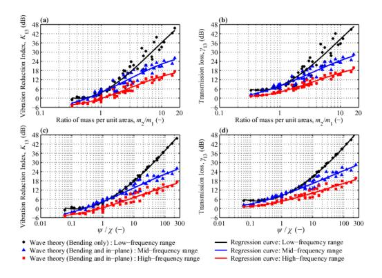
**Figure 5.** Comparison of T-junction data (transmission across the straight section) calculated using wave theory. (a)  $K_{13}$  versus M, (b)  $-10\lg(\gamma_{13})$  versus M, (c)  $K_{13}$  versus  $\psi/\chi$ , (d)  $-10\lg(\gamma_{13})$  versus  $\psi/\chi$ .
