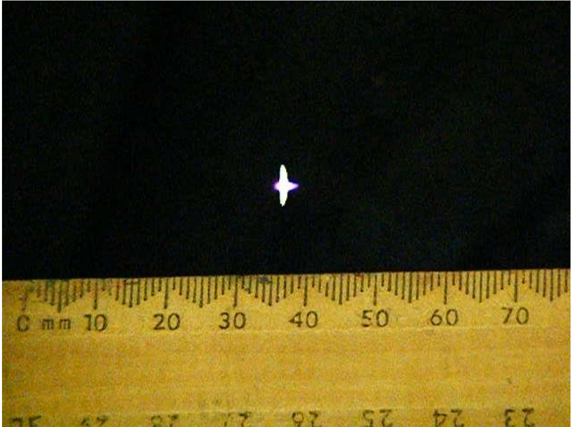
Figure 84. Frame 5342 from a 5 minute video capture showing the cross image phenomenon. A plasma has formed, but the camera was unable to capture an image of the plasma. This frame was taken from a video recorded for a 5 cm focal length lens without frequency doubling.
