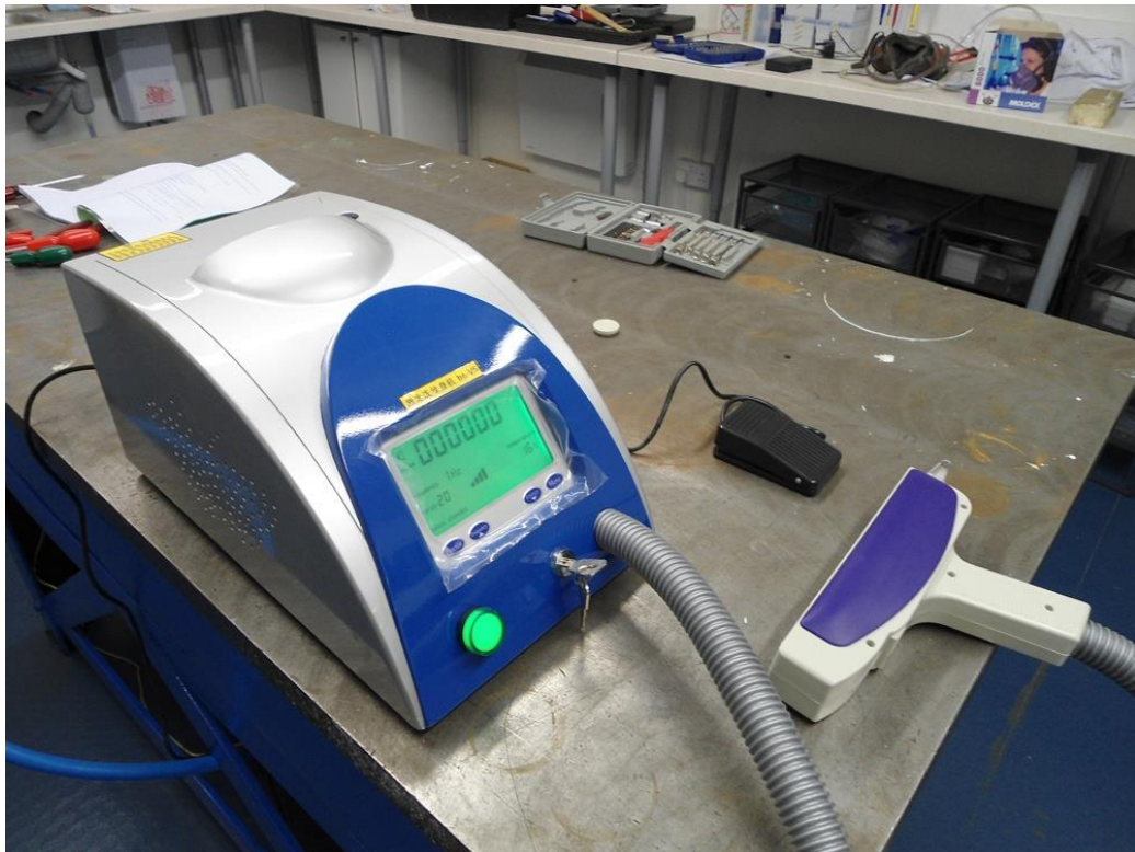
Figure 38. The tattoo removal machine showing the housing for the electronics and water pump. The foot pedal and laser gun are on the right.
