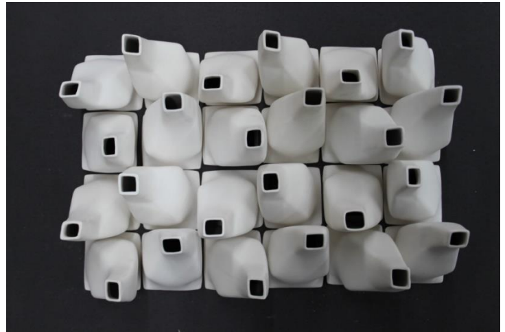
Figure 15: Finalised array of cones after firing
