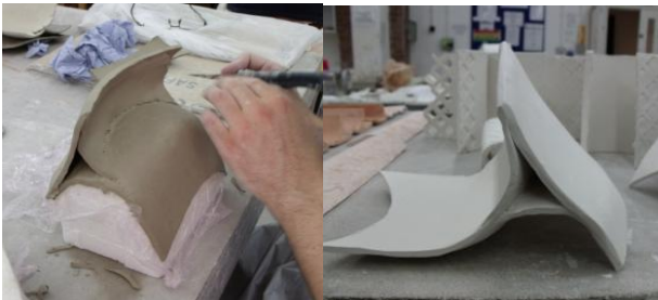
Figure 06: Forming the component out of clay slabs
