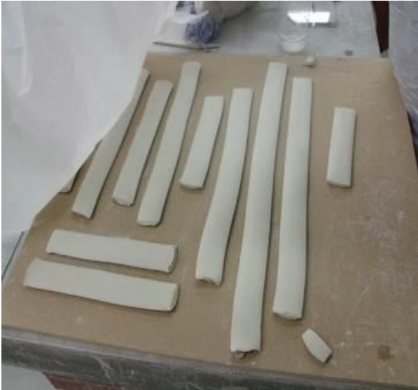
Figure 10: Unformed clay extrusions
