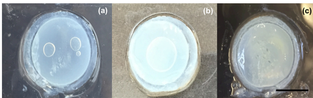
Figure 3.23 Photographs of gel- 1,2 (a) as initially formed (b) after irradiated for 30 minutes and (c) after irradiation for 2 hours under 365 nm LED.
