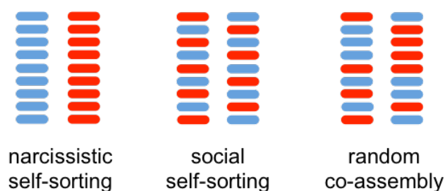
Figure 3.2 The three possible types of co-assembled fibres from a two component system.
