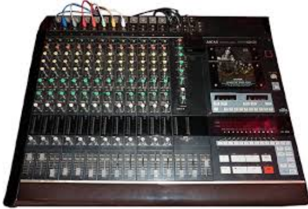
Akai MG1212 digital recorder with built in mixing desk. (Akai MG1212, n.d.)
