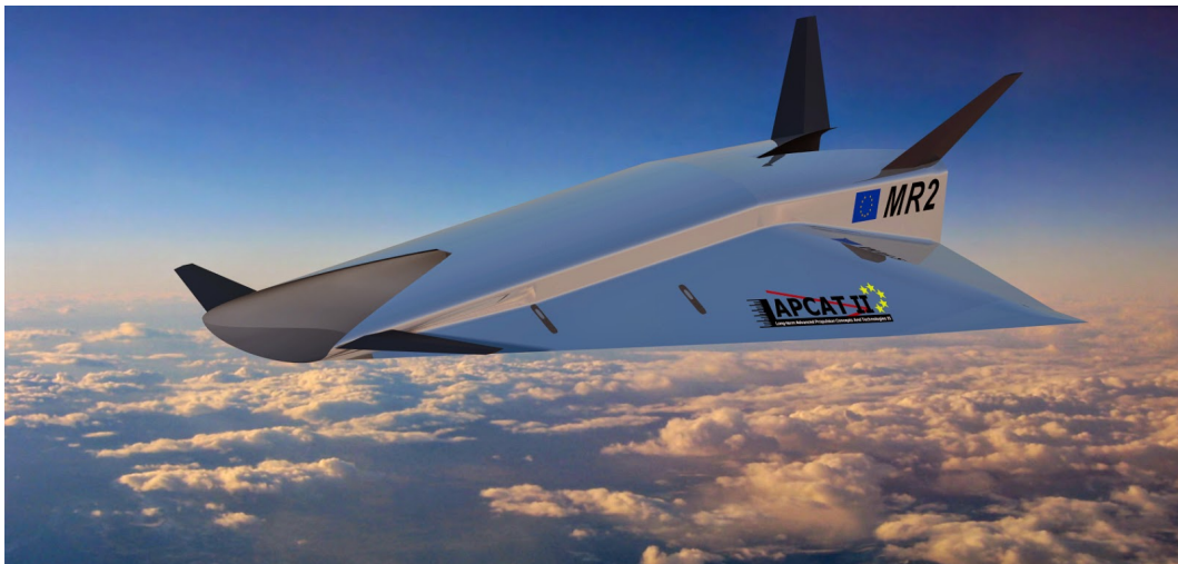
(c) ESA completely integrated vehicle concept for Mach 8 flight, designed in the context of the HEXAFLY [197] and LAPCAT [198] projects.
