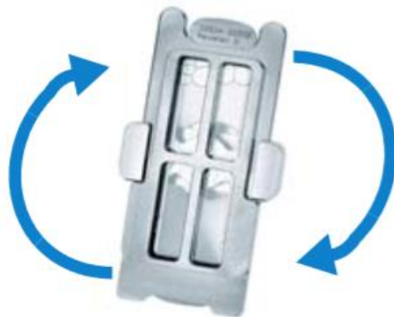
Figure 23| Preparation of the hybridization assembly: Wetting the gaskets, and assessment of bubble mobility The image was adopted by Agilent Technologies ( www.agilent.com ).
