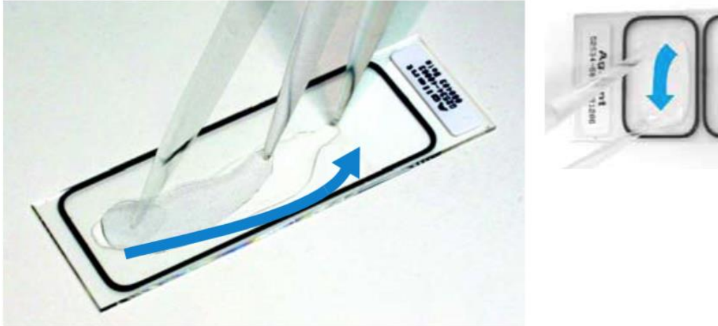
Figure 21| Preparation of the hybridization assembly: “Drag and dispense” of sample The image was adopted by Agilent Technologies ( www.agilent.com ).
