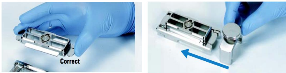
Figure 22| Preparation of the hybridization assembly: Placement of SureHyb onto sandwiched slides The image was adopted by Agilent Technologies ( www.agilent.com ).
