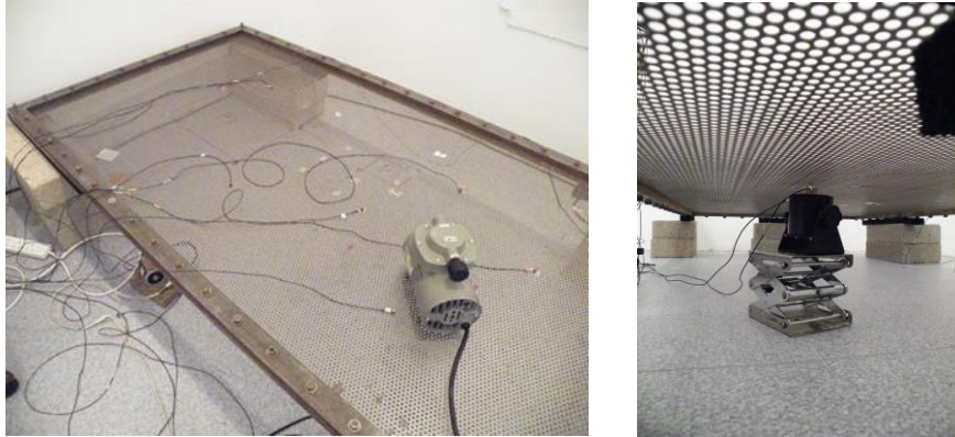
Figure 2. Left: pump attached to the perforated plate with remote accelerometers; right: shaker with inline force transducer for power calibration.
