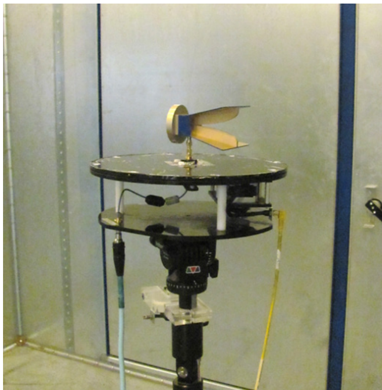
Fig. 5.64. Antenna 2 mounted on a rotation platform as a source stirrer.
