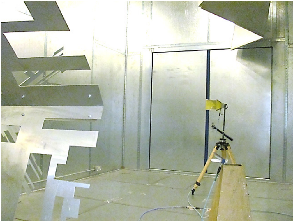
Fig. 1.2. Reverberation chamber at the University of Liverpool.
