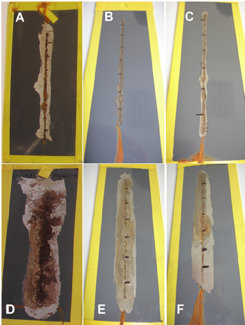
Figure 10 shows two another successful applications of inhibitor loaded halloysite based nanocontainers. Powder coated steel specimens were subjected to a neutral salt spray test (NSS-Test) according to ASTM B117 for 500 hours. As one can see, independently from the chemical composition of the coating matrix, introduction of inhibitor loaded nanocontainers led to significant improvement of anticorrosion performance of the coating both for corrosion development on the scratched site as well as for the extend of delamination around the scratch.
