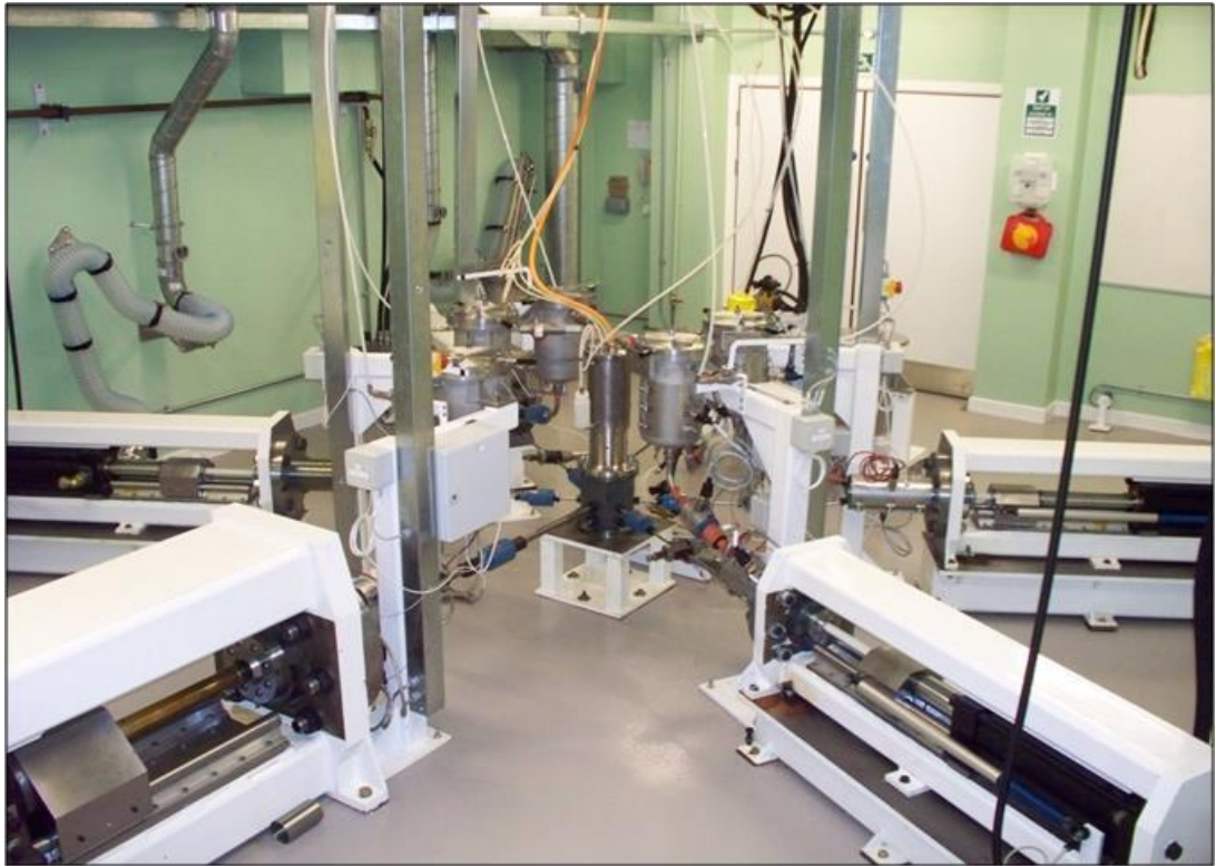
Figure 4.8: Image displaying the CDDM Laboratory system, comprising of 5 feed streams to the central mixer assembly, consisting of a motor, mixing housing and CDDM.
