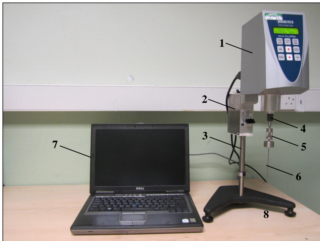
Figure 4.3: Schematic describing the equipment setup for the Brookfield DV-II Pro Extra Viscometer, consisting of an operating panel (1), a moving arm (2), a helipath stand (3), a shipping cap (4), a spindle holder (5), a T-bar spindle (6) and a CPU (7).
