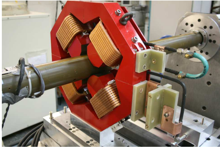
FIGURE B.5: A focusing quadrupole on the rotating coil test bench. The field clamp positions were adjusted in order to give the same integrated field (measured at 35 mm) for all magnets of the given type.
