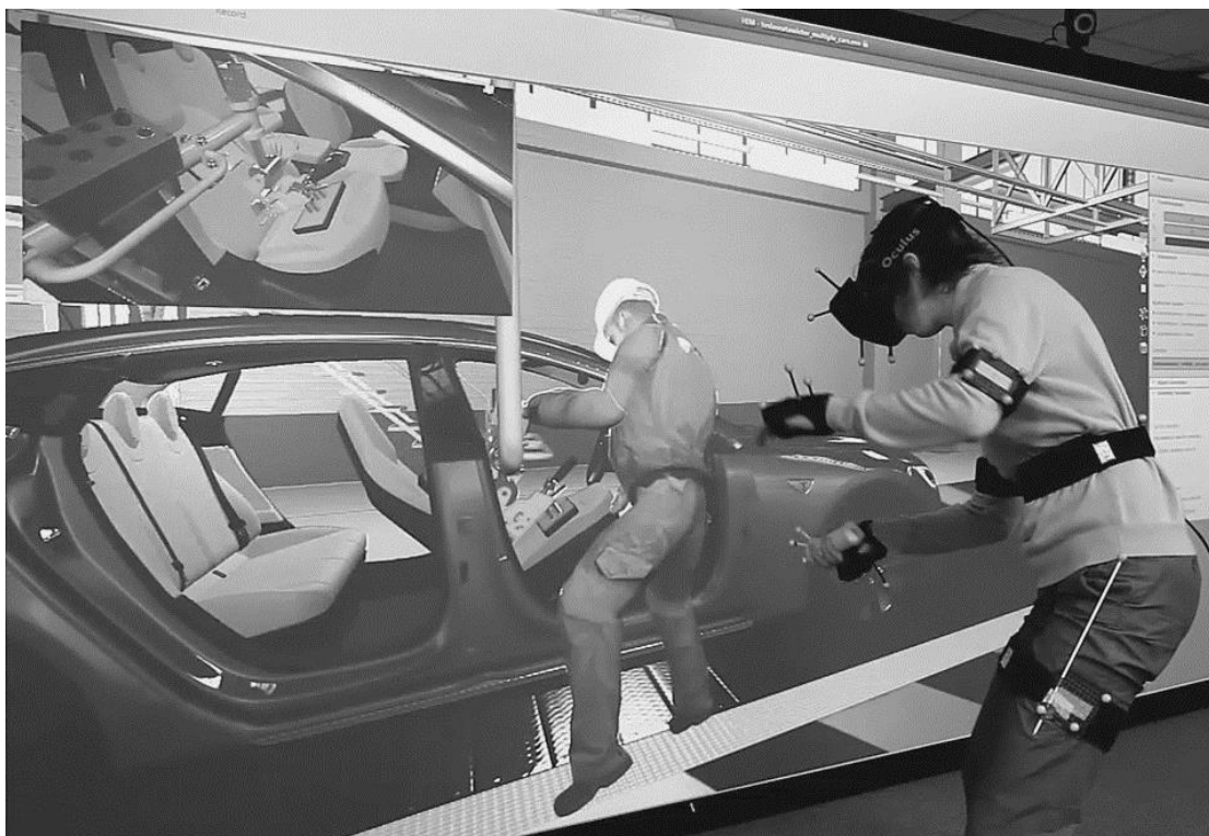
Fig. 5. Simulation of a front-seat assembly using the OPTIS HIM software platform
