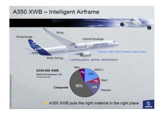
Fig. 1.3 The ratio of materials used in A350 [7]
