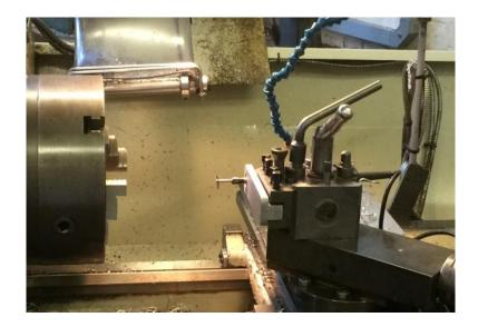
Fig. 3.2 The overview of Dremel, saw and matched mould assembled in lathe
