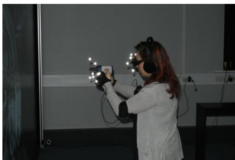
Figure 2. Participant wear headphones, vibration gloves and holding impact wrench whilst performing the task.
