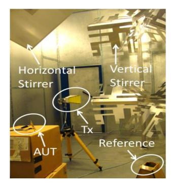
Fig. 2.9: Diversity gain measurement setup in a RC
