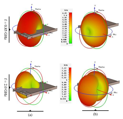
Fig. 7.20: Simulated 3D radiation patterns (a) at 0.85 GHz and (b) at 2.0 GHz
