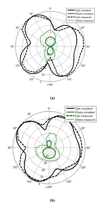
Fig. 3. 23: Radiation patterns in XY plane at 2.5 GHz (a) Feed 1, (b) Feed 2
