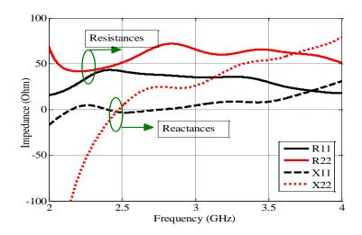
Fig. 4.12: Input impedance as a function of frequency
