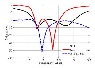
Fig. 4.21: Modified design response for 55 mm  $\times$  100 mm smartphone PCB
