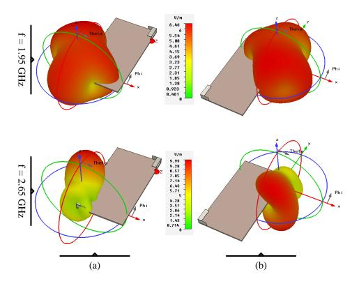
Fig. 5.15: 3D simulated radiation patterns (a) Antenna 1 and (b) Antenna 2
