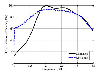
Fig. 5.11: Simulated and measured total radiation efficiency
