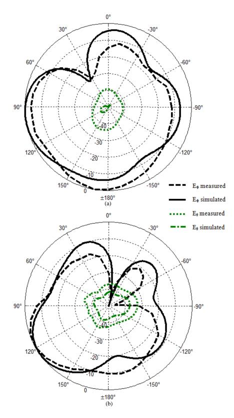
Fig. 5.7 Measured and simulated radiation patterns in XY plane
