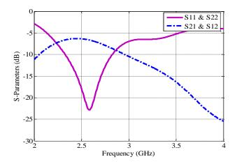
Fig. 3.19: S-parameters of the dual-feed water antenna without the decoupling element
