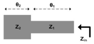
Fig. 6.5: Layout of a conventional two-section quarter wavelength SIR
