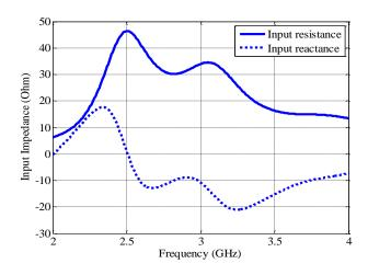
Fig. 3.8: Input impedance of the single feed water antenna
