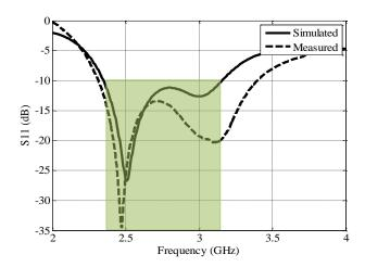
Fig. 3.7: Measured and simulated reflection coefficients
