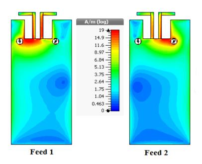
Fig. 3. 20: Surface current distribution at 2.5 GHz
