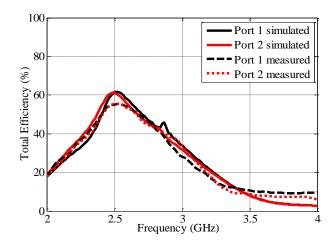
Fig. 3. 27: Measured and simulated total efficiency
