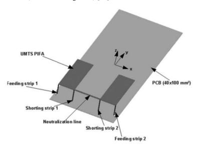
Fig. 2.14: Neutralization line between two PIFA antennas [72].
