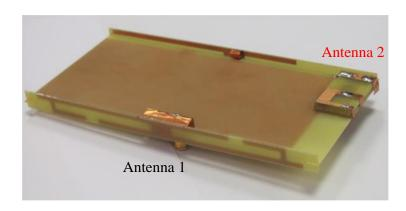
Fig. 7.17: Dual-element antenna prototype
