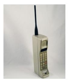
Fig. 1.2: First mobile phone with external Whip antenna
