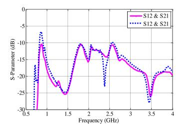
Fig. 7.16: Mutual coupling coefficient before and after modification
