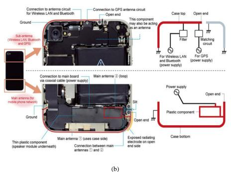
Fig. 1.5: Hybrid antenna (a) Schematic diagram [34] and (b) iPhone 4, the first mobile phone with a metallic frame antenna
