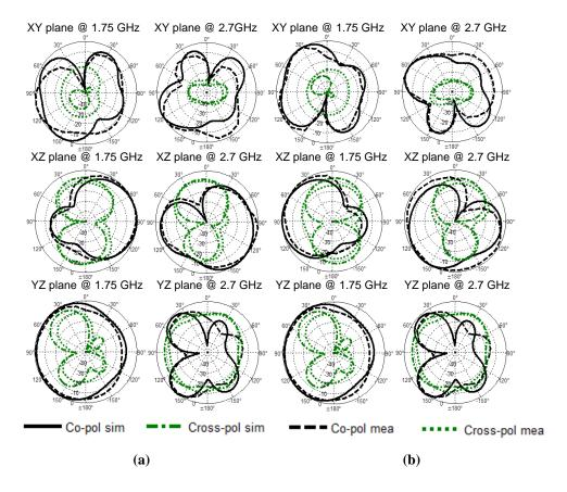
Fig. 6.14: Measured and simulated radiation patterns (a) Element 1 and (b) Element 2
