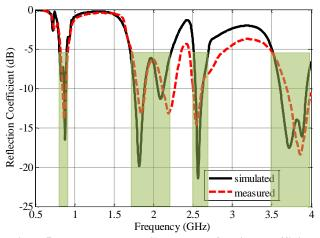
Fig. 7.5: Measured and simulated reflection coefficients
