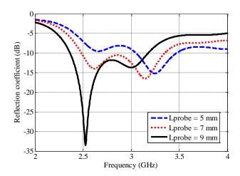
Fig. 3.12: The effect of the probe length
