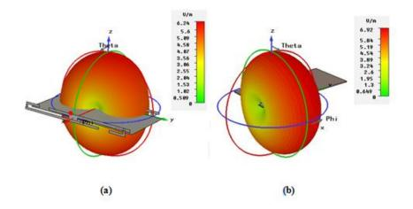
Fig. 7.11: Far field 3D radiation patterns at 0.85 GHz (a) Hexa-band metal frame antenna and (b) Hepta-band PILA antenna
