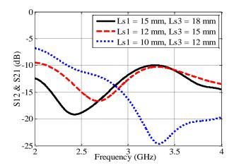
Fig. 4.16: Effect of different L-slot lengths on mutual coupling coefficients
