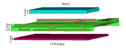
Fig. 7.23: Antenna Configuration with a display and battery
