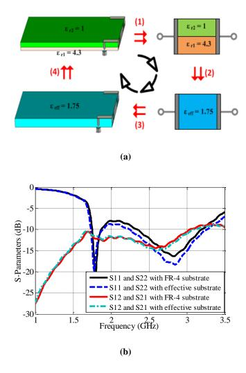
Fig. 6.9: Effective permittivity (a) Parallel capacitance theory and (b) Validation of the calculation
