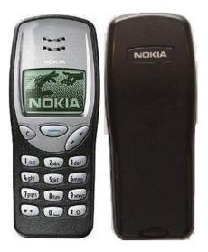
Fig. 1.4: Nokia 3210, the first mobile phone with an internal antenna
