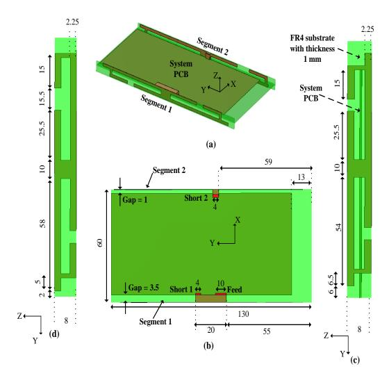
Fig. 7.1: Geometry of the proposed design: (a) 3D antenna geometry, (b) the top view with detailed dimensions, , (c) Segment 1 with detailed dimensions and (d) Segment 2 with detailed dimensions. (Unit: mm)
