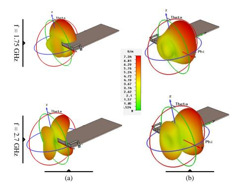
Fig. 6.15: 3D simulated radiation patterns (a) Element 1 and (b) Element 2
