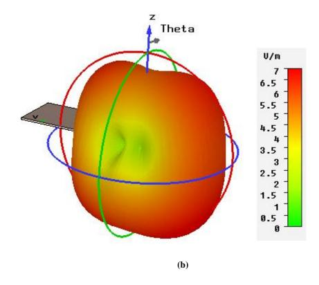
Fig. 4.14: 3D simulated radiation patterns at 2.5 GHz
