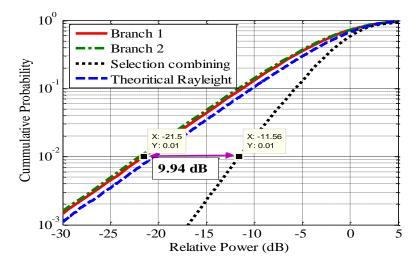
Fig. 4.19: CDF functions and apparent diversity gain
