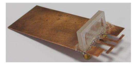
Fig. 3.17: Dual-feed water antenna prototype
