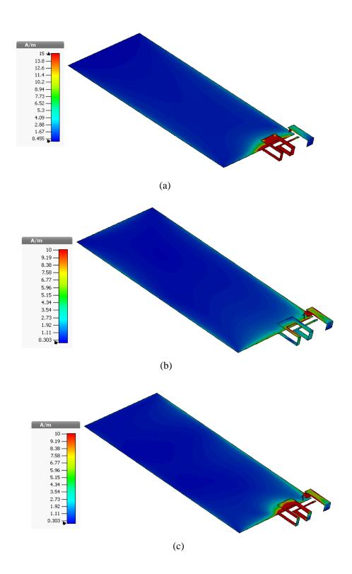
Fig. 7.10: Simulated surface current distributions (a) f = 0.85 GHz,
