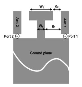
Fig. 6.7: General geometry of dual-element monopole antenna with a parasitic decoupling element
