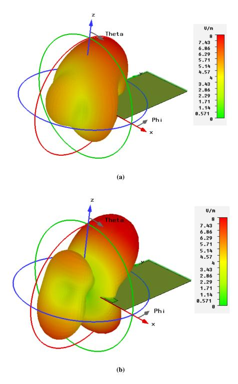
Fig. 5.10: 3D simulated radiation patterns (a) at 1.95 GHz and (b) at 2.64 GHz
