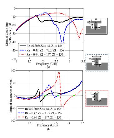
Fig. 6.10: Effect of changing  $\mathbf{Z}_2$  (a) mutual coupling coefficient and (b) mutual coupling impedance
