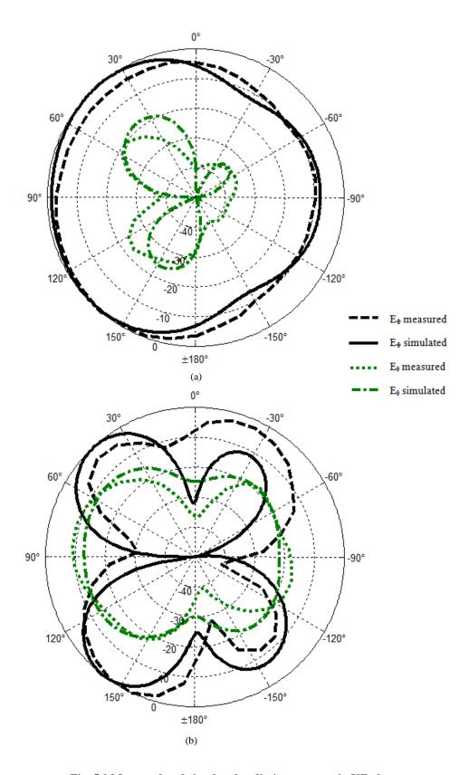
Fig. 5.9 Measured and simulated radiation patterns in YZ plane
