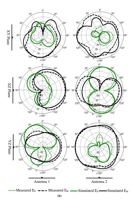
Fig. 7.19: Normalized far-field radiation patterns (a) at 0.85 GHz and (b) at 2.0 GHz
