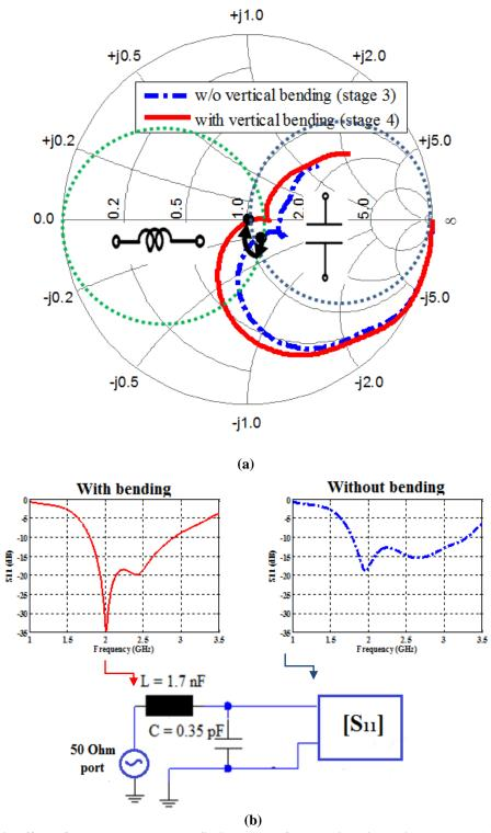
Fig. 5.3. Effect of the bended plate (a) Smith chart of normalized input impedance, (b)  $S_{11}$  and equivalent matching circuit
