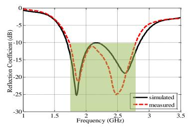
Fig. 5.6: Measured and simulated reflection coefficients of single element
