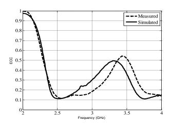
Fig. 3. 25: Measured and simulated envelope correlation coefficient
