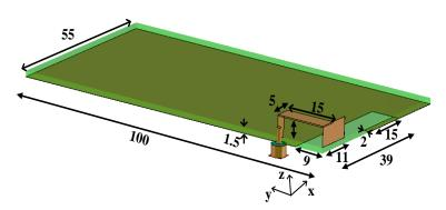
Fig. 5.1: Geometry of the proposed element antenna (unit: mm)
