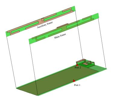
Fig. 7.12: Dual-element multiband antenna design
