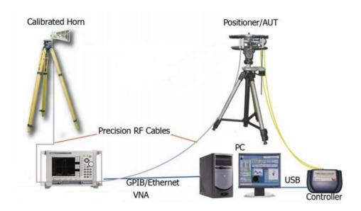
Fig. 2.11: Typical measurement layout.
