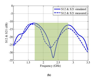
Fig. 5.13 Simulated and measured S-parameters (a) Reflection parameters and (b) isolation parameters
