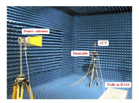
Fig. 2.10: The anechoic chamber at the University of Liverpool
