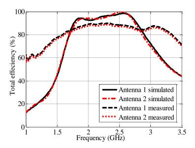
Fig. 5.18: Total efficiency of the proposed antenna
