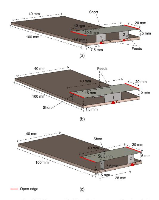
Fig. 4.1: PIFA antenna with different feed arrangements (a) coplanar feed, (b) parallel feed and (c) orthogonal feed
