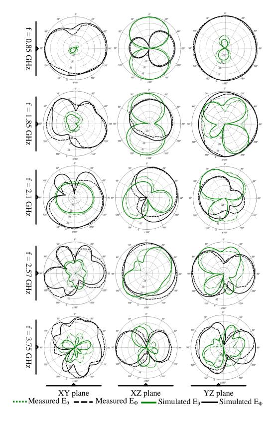
Fig. 7.6: Simulated and measured normalized far field radiation patterns
