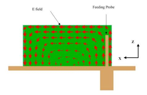
Fig. 3.4: Coaxial probe feed coupling for  $TE_{1\delta 1}^{y}$  RDRA mode
