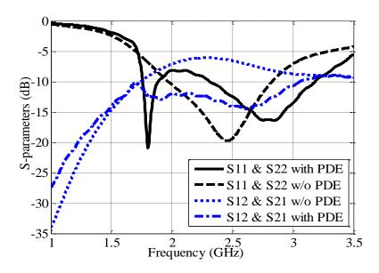
Fig. 6.2: Simulated scattering parameters (PDE: mean, parasitic decoupling element).
