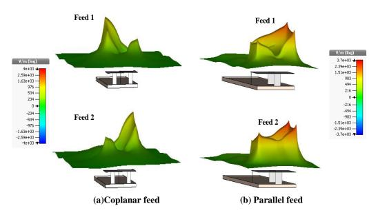
Fig. 4.3: Electric field distributions on top plate at 2.5 GHz (a) coplanar feed and (b) parallel feed
