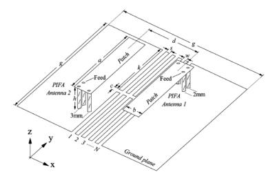
Fig. 2.13: Isolation using DGS structure [68].
