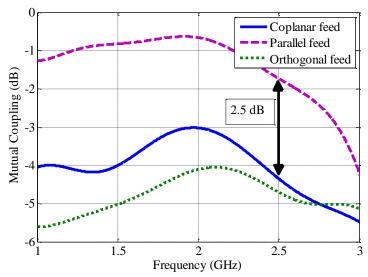
Fig. 4.2: Mutual coupling between PIFA feeds
