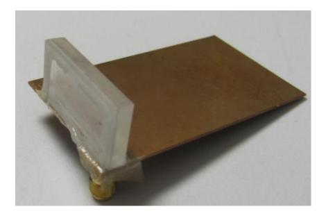
Fig. 3.6: Single-feed water-based antenna prototype
