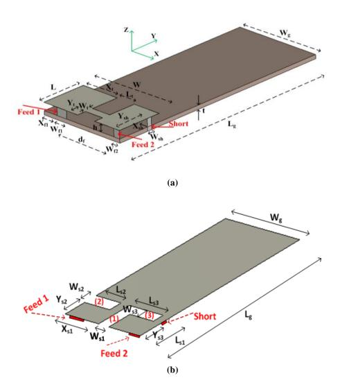
Fig. 4.7: Structure of dual-coplanar feed PIFA antenna (a) structure and (b) modified ground plane
