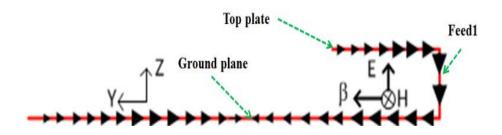
Fig. 4.6: Side view of dual-coplanar-Feed PIFA over ground plane with surface current distribution and excited fields between parallel plates at 2.5 GHz
