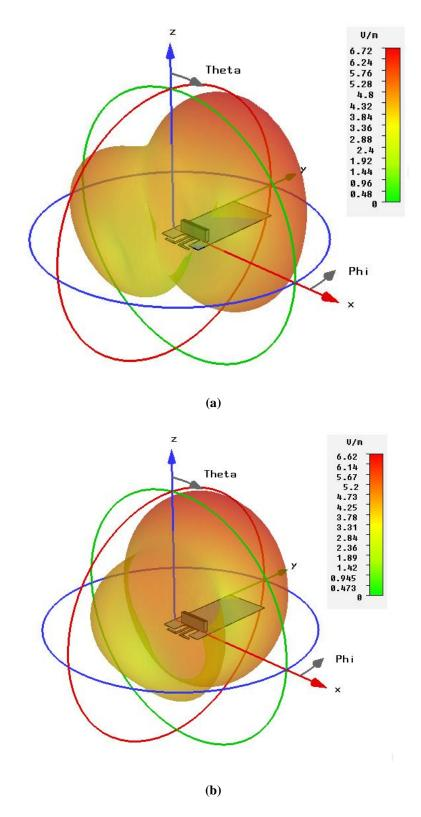
Fig. 3. 24: Simulated 3D radiation patterns at 2.5 GHz (a) Feed 1, (b) Feed 2
