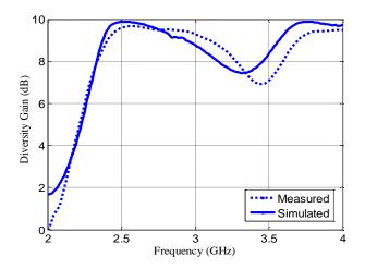
Fig. 3. 26: Measured and simulated diversity gain using ECC
