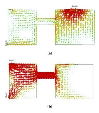
Fig. 4.11: Directions of currents on the top plate at 2.5 GHz (a) Feed 1 and (b) Feed 2
