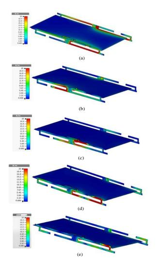
Fig. 7.3: Simulated surface current distributions (a) 0.85 GHz, (b) 1.85 GHz, (c) 2.1 GHz, (d) 2.55 GHz and (e) at 3.75 GHz.
