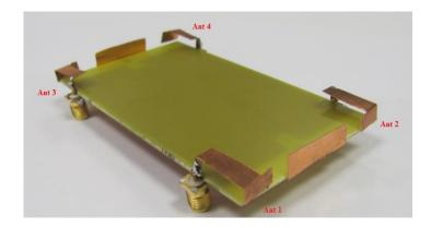
Fig 6.19: Four-element PILA prototype
