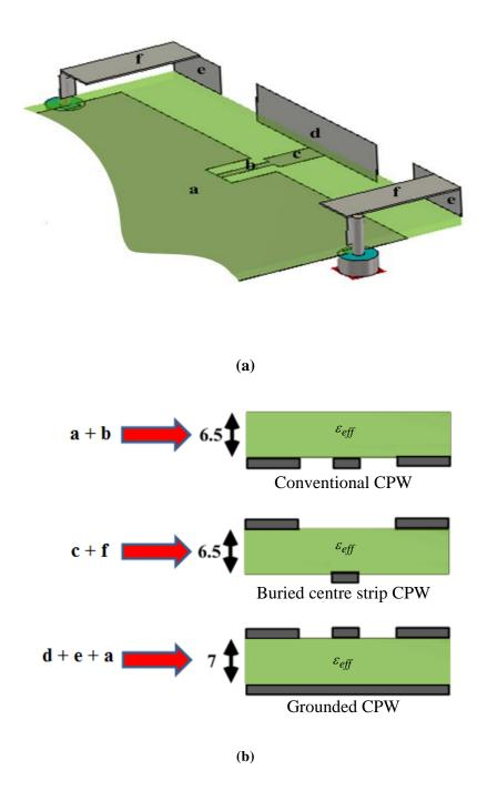
Fig. 6.8: Equivalent CPWs from the proposed structure(a) Proposed structure and (b) the equivalent CPW schemes
