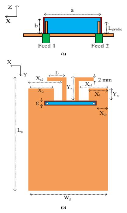
Fig. 3.16: Geometry of the dual-feed water antenna: (a) side view, (b) top view
