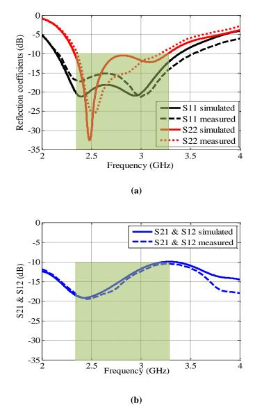
Fig. 4.9: Measured and simulated S-parameters (a) Reflection coefficients, (b) Transmission coefficients
