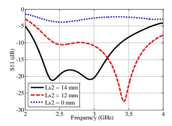
Fig. 4.15: Effect of Slot 2 length on  $S_{11}$ .
