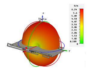
Fig. 7.7: 3D simulated far field pattern at 0.85 GHz
