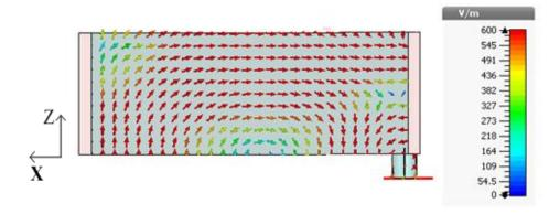
Fig. 3.9: Electric field distribution of the excited  $TE_{1\delta 1}^y$  mode at 2.5 GHz
