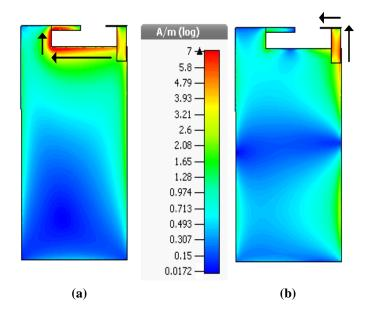
Fig. 5.4: Simulated surface current distributions (a) at 1.95 GHz and (b) at 2.64 GHz
