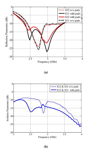
Fig. 3. 22: Effect of the added ground plane pads (a) S11 and S22, (b) S21 and S12
