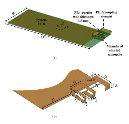
Fig: 7.8: Antenna configuration (a) Whole configuration and (b) Detailed dimensions (unit: mm)
