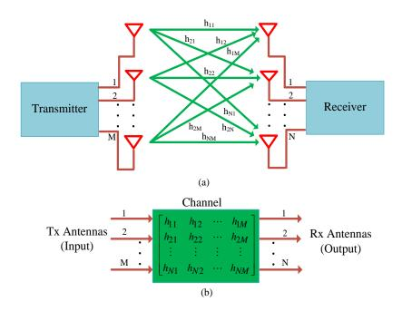
Fig. 2.2: (a) Multiple input multiple output (MIMO) system and
