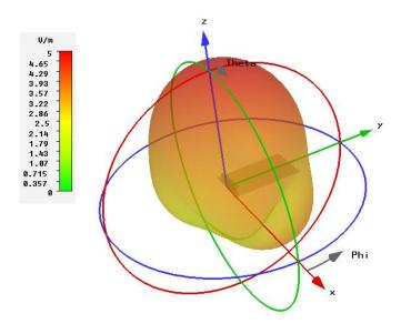
Fig. 3.13: 3D simulated far field radiation pattern at 2.5 GHz
