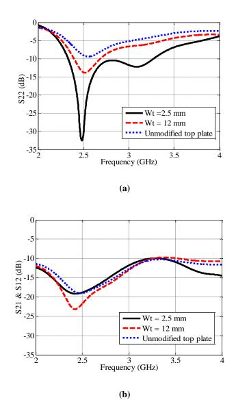
Fig. 4.17: Effect of top plate strip width on (a) Reflection coefficient of Feed 2 and (b) Mutual coupling coefficient
