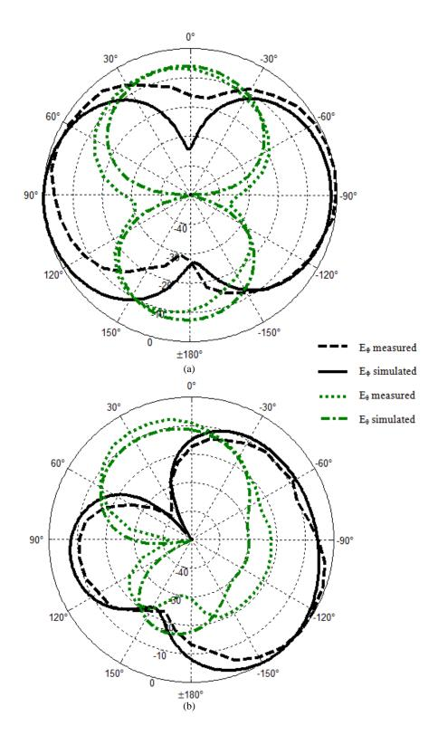
Fig. 5.8 Measured and simulated radiation patterns in  $\boldsymbol{X}\boldsymbol{Z}$  plane
