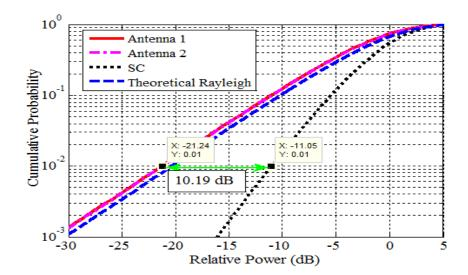
Fig. 5.17: CDF functions and apparent diversity gain
