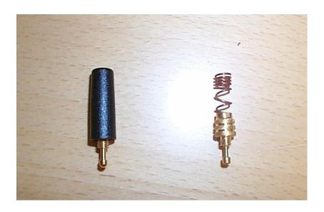
Fig. 1.3: Dual band non-uniform helix antenna invented by Z. Ying [10].
