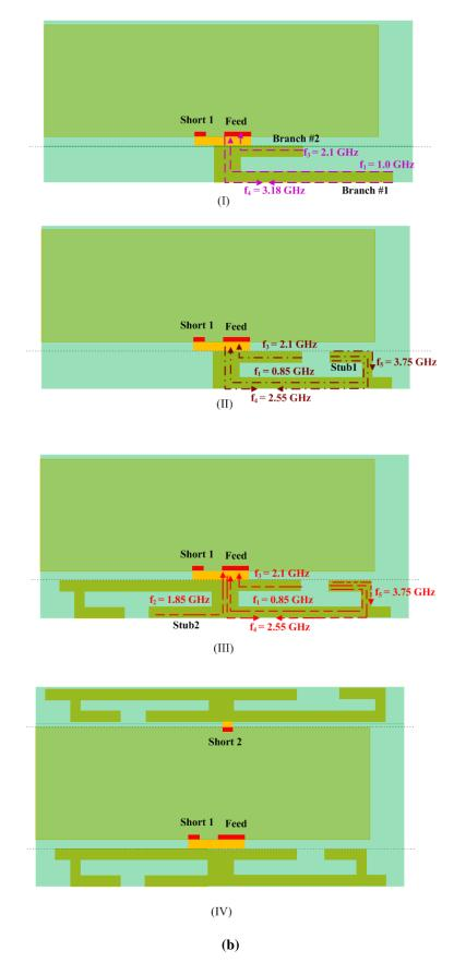
Fig. 7.2: (a)  $S_{11}$  evolutions, (a) the step by step change on the frame geometry (planar form)
