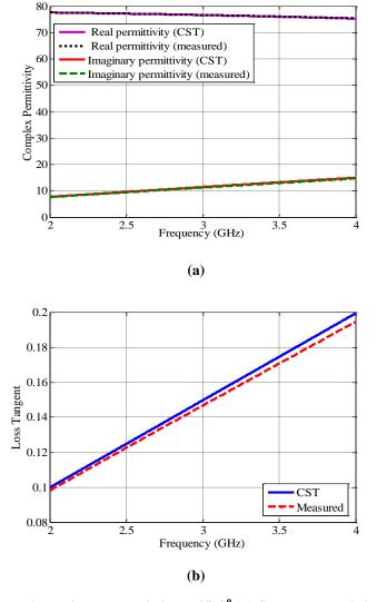
Fig. 3.1: Pure water dielectric characteristics at 25  $C^0$  (a) Complex permittivity (b) Loss tangent
