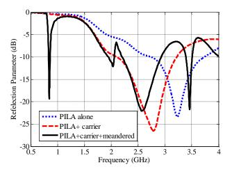
Fig. 7.9: Reflection coefficient evolutions
