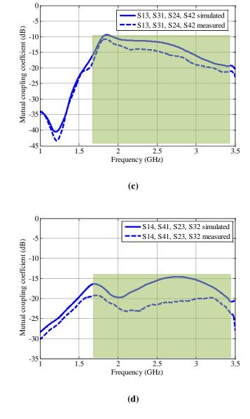
Fig. 6.20: Measured and simulated S-parameters (a) Reflection coefficients, (b), (c) and (d) Mutual coupling coefficients
