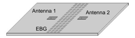
Fig. 2.12: EBG structure between two microstrip antennas [67].
