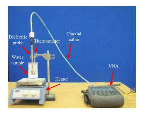
Fig. 3.2: Complex permittivity measurement setup
