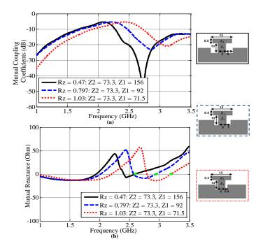
Fig. 6.11: Effect of changing  $\mathbf{Z}_1$  (a) mutual coupling coefficient and (b) mutual coupling impedance
