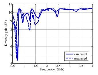
Fig. 7.22: Apparent diversity gain versus frequency
