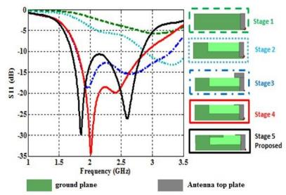
Fig. 5.2: The step by step change on geometry and  $S_{11}$  evolutions
