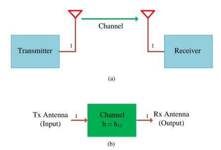
Fig. 2.1: (a) Single input and single output (SISO) system and (b) SISO from channel perspective
