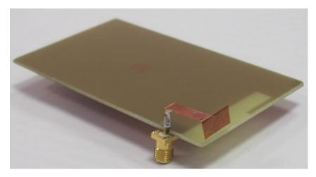
Fig. 5.5. Single element PILA prototype
