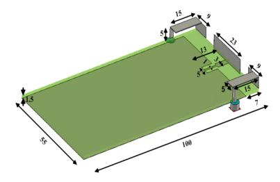
Fig. 6.1: The proposed dual-element antenna with dimensions in [mm].
