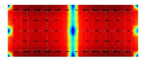
Fig. 4.5: Characteristic mode of a rectangular 40 mm  $\times 100$  mm ground plane computed at 2.5 GHz [23].
