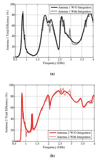
Fig. 7.25: Effect of the LCD display and battery models on the total efficiencies (a) Antenna 1 (metal frame) and (b) Antenna 2 (PILA with meandered strip monopole)
