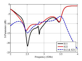
Fig. 3. 28: S-parameters of the proposed dual-feed RDRA antenna with a loss-free material having a dielectric constant  $\, {\cal E}_r = 81 \,$
