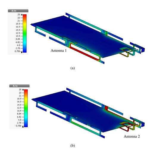
Fig. 7.14: Simulated surface current distribution at 0.85 GHz
