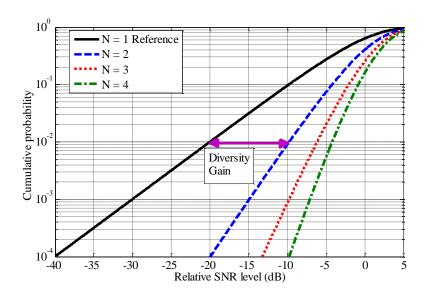
Fig. 2.5: Cumulative distribution functions of relative SNR threshold
