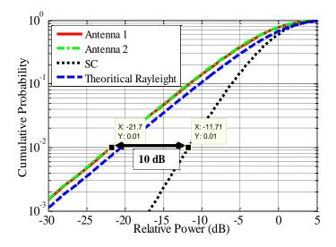
Fig. 6.17: CDF function and measured apparent diversity gain
