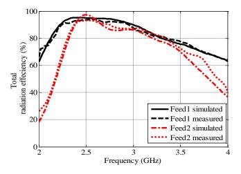
Fig. 4.20: Measured and simulated total efficiency
