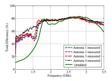
Fig. 6.24: The total radiation efficiency
