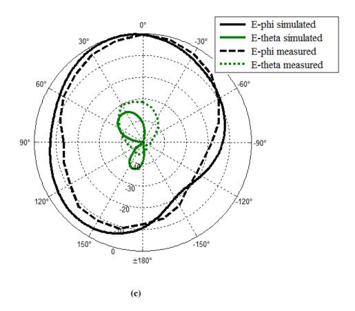
Fig. 3.14: Measured and simulated radiation patterns at 2.5 GHz
