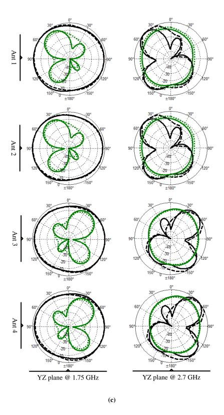
Fig. 6.21: Measured and simulated far-field normalized radiation patterns (a) XY plane (b) XZ plane and (c) YZ plane (Black  $E_{\phi}$ , Green  $E_{\theta}$ , the solid lines represent the simulated results, while the dashed and dotted lines are the measured patterns)
