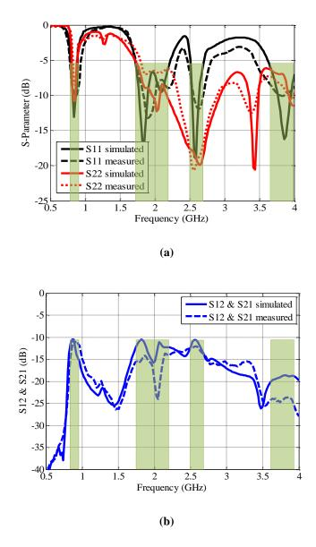
Fig. 7.18: Simulated and measured S-parameters
