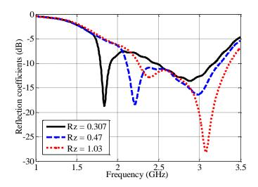
Fig. 6.12: Effect of changing impedance ratio on the reflection coefficients
