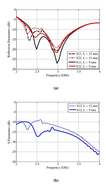
Fig. 3. 21: Effect of L-shaped strip length (a) S11 and S22, (b) S21 and S12
