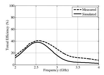
Fig. 3.15: Measured and simulated total efficiency
