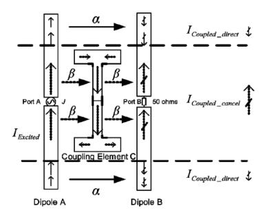
Fig. 2.15: Isolation using parasitic decoupling element [75].
