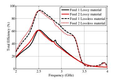
Fig. 3. 29: Radiation efficiency comparison between RDRA with a lossless material of  $\varepsilon_r=81$  and a lossy material of  $\varepsilon_r=81$
