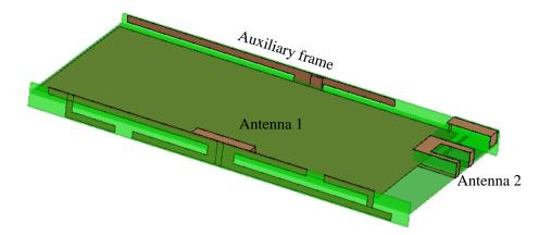
Fig. 7.15: Final configuration after modifying the auxiliary frame
