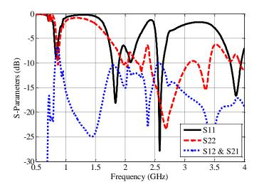
Fig. 7.13: Initial simulated S-parameters versus frequency in GHz
