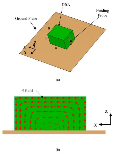
Fig. 3.3: Rectangular dielectric resonator antenna(a) RDRA antenna, (b) Electric field lines of the fundamental mode ( $TE_{1\delta 1}^y$ )
