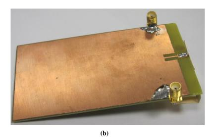
Fig. 6.3: Prototype of the proposed antenna (a) top view and (b) back view
