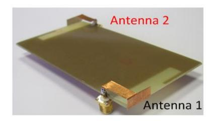
Fig. 5.12: Dual-element PILA Antenna
