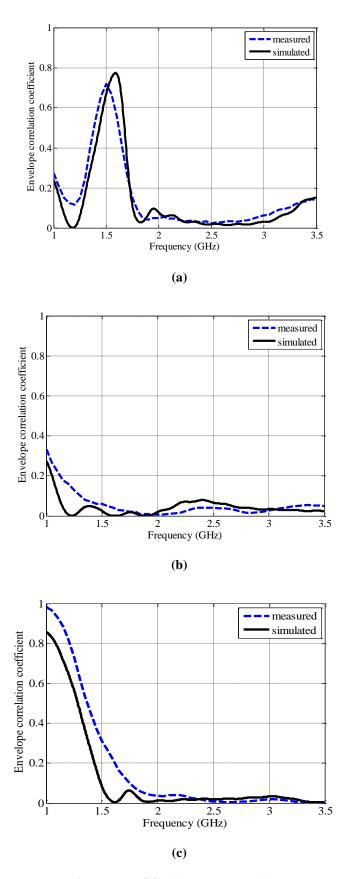
Fig. 6.22: Measured and simulated ECCs (a)  $\rho_{12}$ ,  $\rho_{34}$ ; (b)  $\rho_{13}$ ,  $\rho_{24}$  and (c)  $\rho_{14}$ ,  $\rho_{23}$
