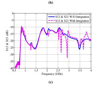
Fig. 7.24: Variation of the S-parameters of the antenna when including the LCD display and battery models (a)  $S_{11}$ , (b)  $S_{22}$  and (c)  $S_{12}$  and  $S_{21}$
