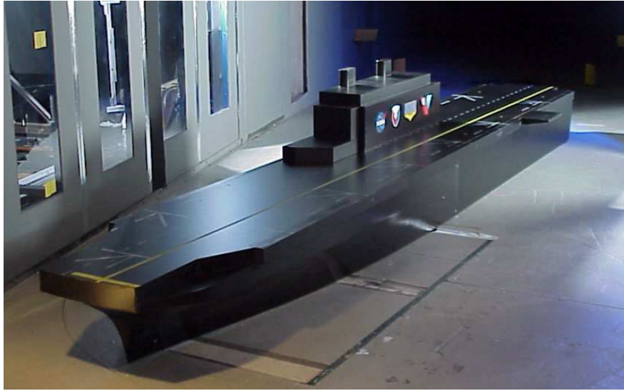
Figure 1.22: Model of the Landing Helicopter Assault ship (LHA) used at NASA Ames Research Center
