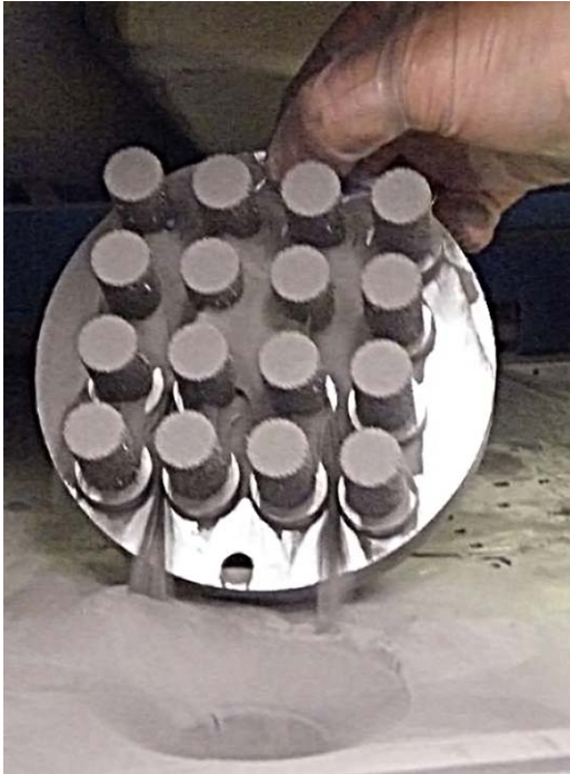
FIGURE 1. Sixteen test cylinders on a substrate holder showing surplus Ti powder pouring off at the end of the manufacturing process. [Color figure can be viewed in the online issue, which is available at wileyonlinelibrary.com .]
