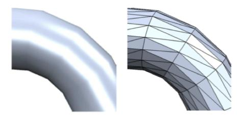
FIGURE 2.10: Triangular mesh representation using j = 3 [134].
