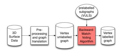
FIGURE 6.1: Schematic for predicting vertex labels given a new 3D surface data set.
