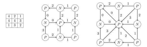
FIGURE 3.11: Grid representation with "Z" values (left), with corresponding grid graph where degree=4 (middle) and cross-grid graph where degree =8 (right), featuring "slope" labels on edges.
