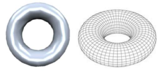
FIGURE 2.11: Rectangular mesh representation using j = 4 [134].
