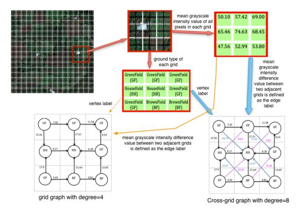
FIGURE 3.13: Process of Translating a satellite image into a "grid graph" and a "crossgrid graph" (the edge colour encoding is for ease of understanding only).
