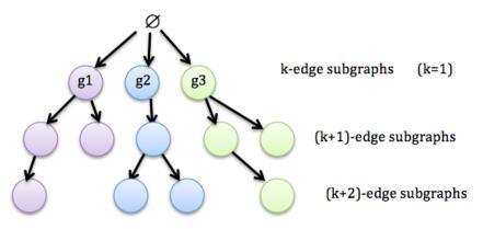
FIGURE 2.9: Pattern-growth (DFS). Only frequent K-edge subgraphs will be grown to (K + 1)-edge subgraphs.
