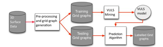
FIGURE 1.3: The VULS mining evaluation process using training and test sets
