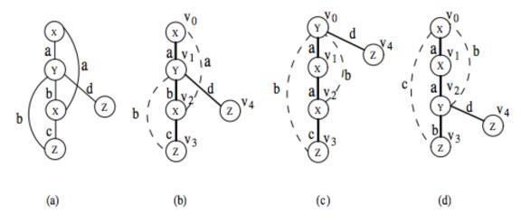
FIGURE 2.3: Depth-First Search Tree and its Forward/Backward Edge Set [229]. Note that forward edges are represented by solid lines and backward edges dashed lines.
