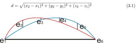
FIGURE 3.7: Cross section at a grid line showing simple vertical springback error calculation between a before (blue line) and an after (red line) shape [129].
