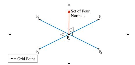
FIGURE 3.8: Error calculation using the line-plane intersection method [129].
