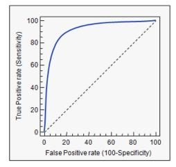
FIGURE 2.13: The ROC curve. The solid blue line indicates a good ROC curve that reaches the upper left corner and the dotted line indicates a random classifier (guessing).
