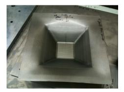
FIGURE 3.3: Square based pyramid (upside down) at the point when it is unclamped after application of the AISF process.
