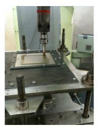
FIGURE 3.2: Example AISF machine 2, a metal sheet is clamped into a holder and the desired shape is produced using the continuous movement of a simple roundheaded forming tool.
