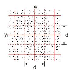
FIGURE 3.6: Coordinate cloud points associated with a grid representation centred on  $\langle x_i, y_j \rangle$  (grid spacing = d) [129].
