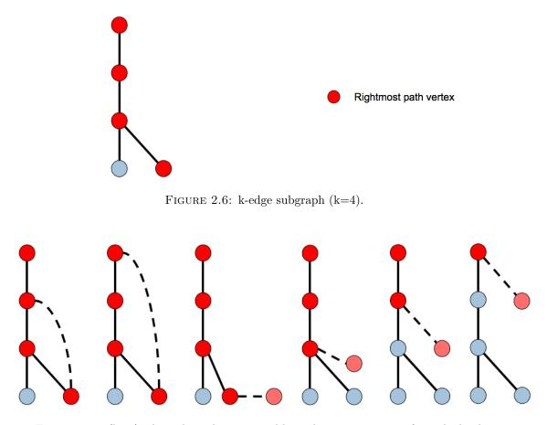
FIGURE 2.7: (k+1)-edge subgraphs generated by right most extension from the k-edge subgraph given in Figure 2.6.
