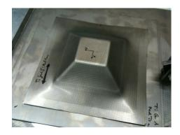
FIGURE 3.4: Square based pyramid (right way up); the markings are used with respect to the GOM optical measuring tool.
