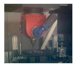
FIGURE 3.1: Example AISF machine 1 [129], the work piece is clamped in position while the tool head "pushes out" the desired shape; on release, springback occurs as a result of which the final shape is not the desired shape.
