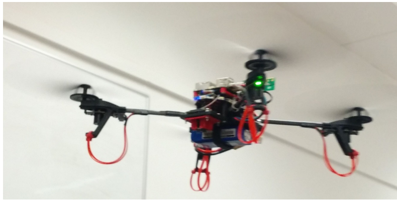
Fig. 2. AR. Drone/PX4-based MAV Platform
