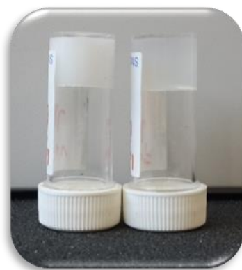
Figure 3.3: Examples of hydrogel images that formed a turbid and transparent gel. Compound 17 (Left) formed a turbid gel and compound 12 (Right) formed a transparent using the GdL method. It shows the effect of the molecular structure on the turbidity.
