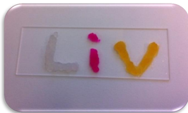
Figure 5.2: an example of image of injectable hydrogel loaded dyes using DMSO: Water method. The gels were prepared in a syringe and then injected on to a microscope slide through a needle.
