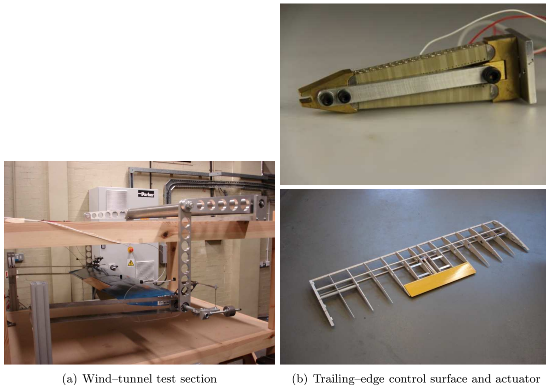
Figure 4.4: Schematic view of the experimental setup of the aeroelastic model at the University of Liverpool
