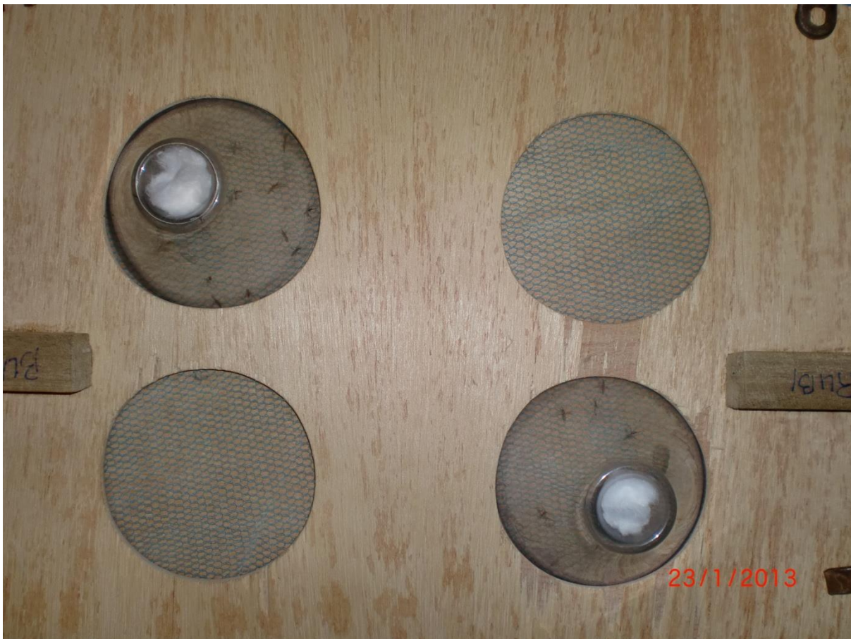
Figure 6.2: Laboratory testing of the nets using WHO cones on one site of the net. Around ten mosquitoes were introduced into the cone and removed after 3 minutes of contact with the net (Lab CNRFP, Ouagadougou) (photo of K.H. TOE).
