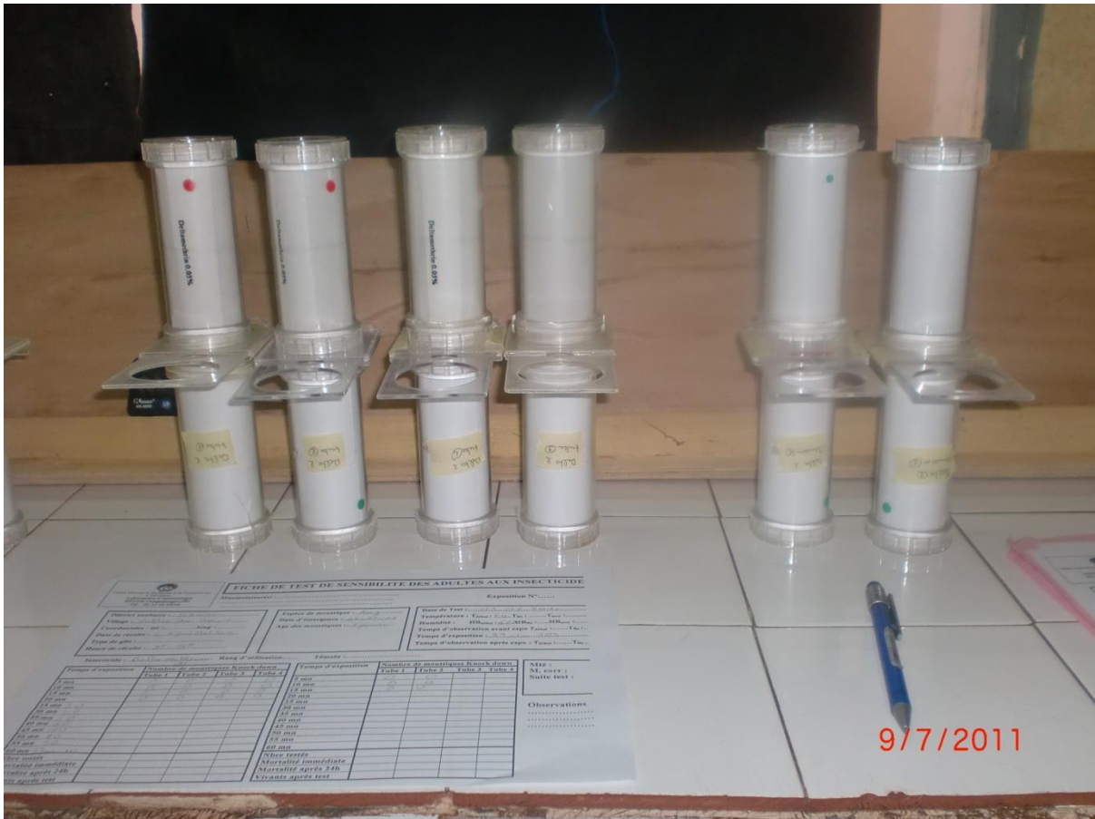
Figure 3.5: bioassays using the WHO tubes protocol, tube labelled in red (top): insecticide exposure tubes, tubes labelled in green (bottom and right): observation tube. All the tubes were in vertical position (photo of K.H TOE).
