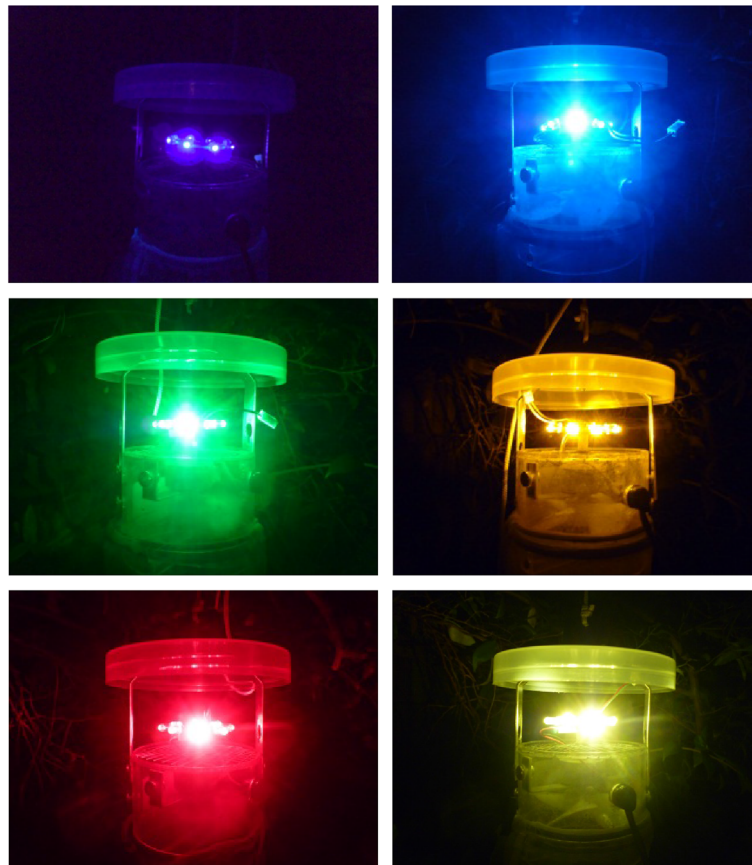
Figure 1 Light emitting diode baits used during investigation of differential attraction of Culicoides to commercially produced light-suction traps. Colours used were: UV (390 nm), Blue (430 nm), Green (570 nm), Yellow (590 nm), Red (660 nm) and White (427-750 nm).
