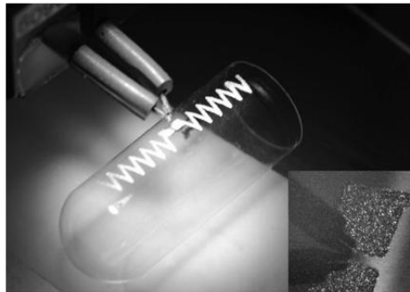
Fig. 2.50: The Zigzag antenna in [73] printed directly onto surface of 00 size gelatin capsule.
