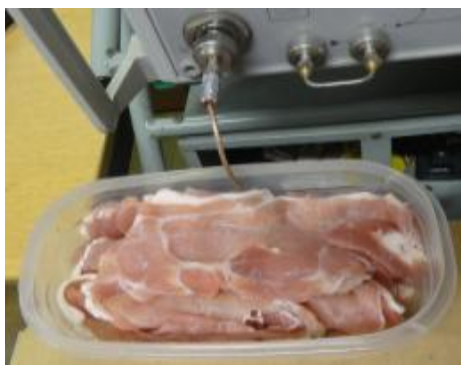
Fig. 3.19: Body phantoms of measurements: (a) The liquid body model (b) Pork Piece 1 and Piece 2, respectively.
