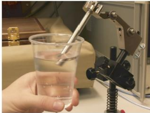
Fig. 2.55: An example illustrates the measurement of liquid body phantom dielectric properties [3]
