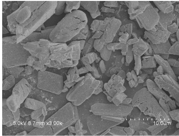
Fig. S3. The SEM image of the bulk ceria sample.
